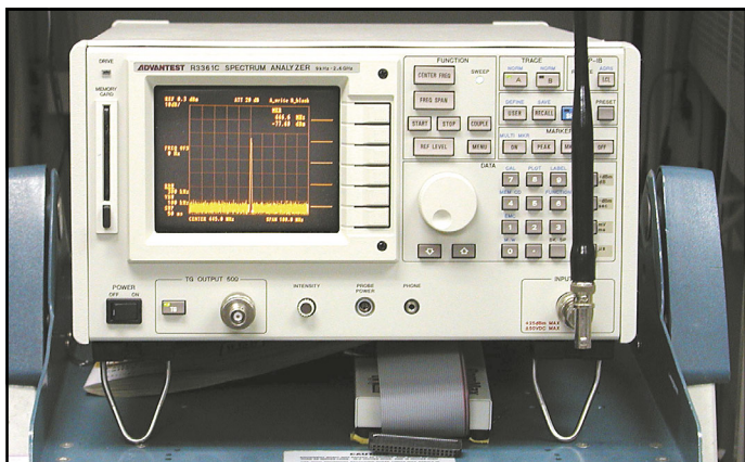
Figure 4—The Advantest R3361C spectrum analyzer used in the test.
